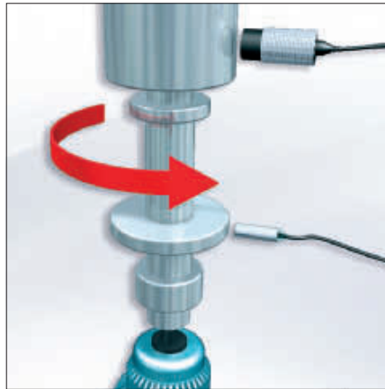
Eccentricity control of a rotating shaft
