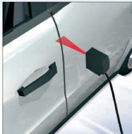
Precise gap measurement in automotive industry
