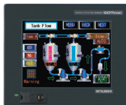
The GOT1000 is a typical HMI.
