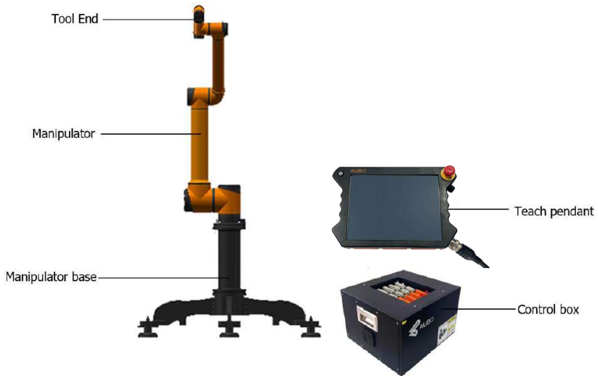
Figure 5-1 AUBO – i10 robot system
