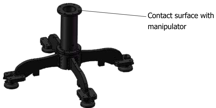
Figure 6-3 Diagram of manipulator base structure
