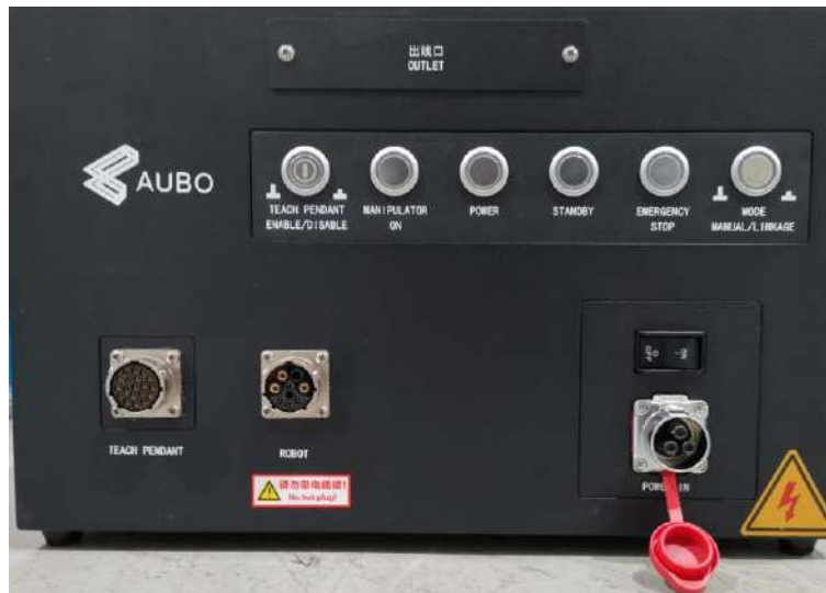
Figure 7-2 Front panel of the control box
