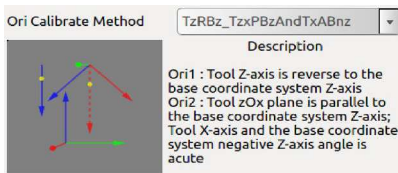
Figure 10-35 TzRBz_TzxPBzAndTxABnz type calibration method
